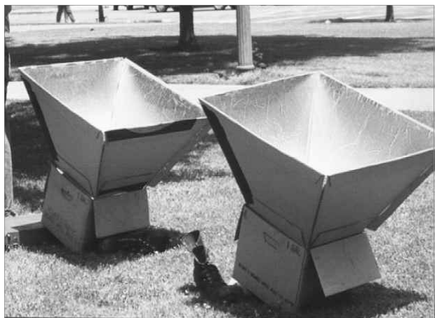
Figure 12.2: Joe Radabaugh's Heaven's Flame multi-reflector solar box cooker, Solar Cookers International
