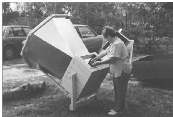
Figure 12.1: The Casa Juliana solar cooker, designed by David Omick, reaches temperatures above 400°F, Andy McDonald
