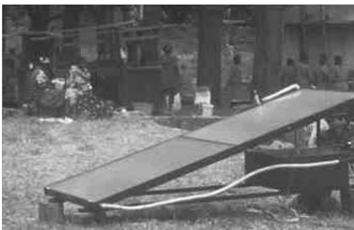
Figure 12.15: Solar water pasteurizer Safe Water Systems
