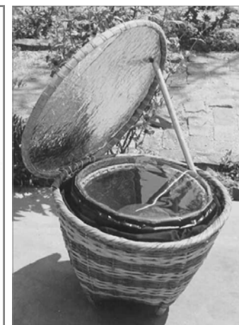
Figure 12.11: A basket cooker at the Centre for Rural Technology in Nepal. Solar Cookers International
