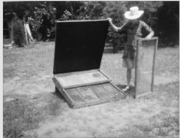
Figure 12.18: Mark Schimmoeller with his solar food dryer, Chris Schimmoeller
